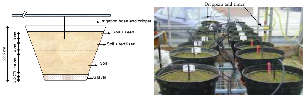
Figure 1: Diagram of a pot (left) and pots with established grass and irrigation system (right).
